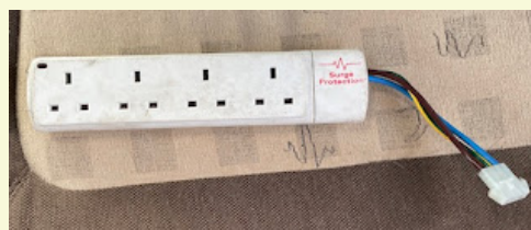
Old PDU connector fitted to mains extension
