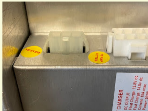
Mains connector in the old PDU
